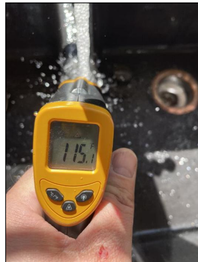
Water temp. at the kitchen faucet. 115 was the best temperature, despite the water heater being set to 140 degrees.
